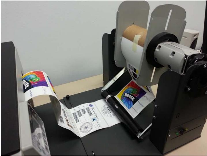
8. Manually rewind the stock onto the core.
