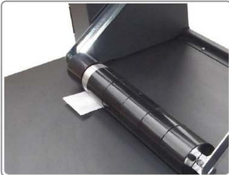
4. Insert a straightened paperclip into the hole on the side with the power switch and two LEDs. This will engage a button inside the rewinder. Keep the button pressed and turn on the device. The yellow LED will be flashing. Remove the clip.
