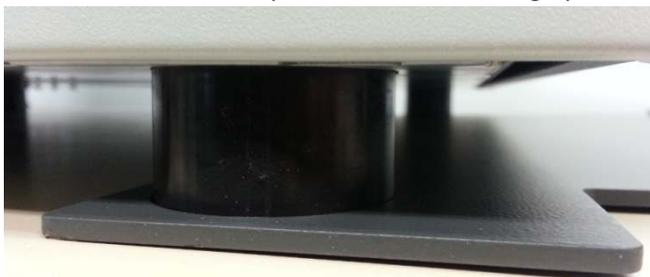
2. Place rewinder on top of base plate, aligning standoffs with the slots in rewinder base plate
