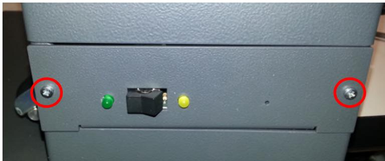
4. Once the screws have been removed, move the power switch plate out of the way.
