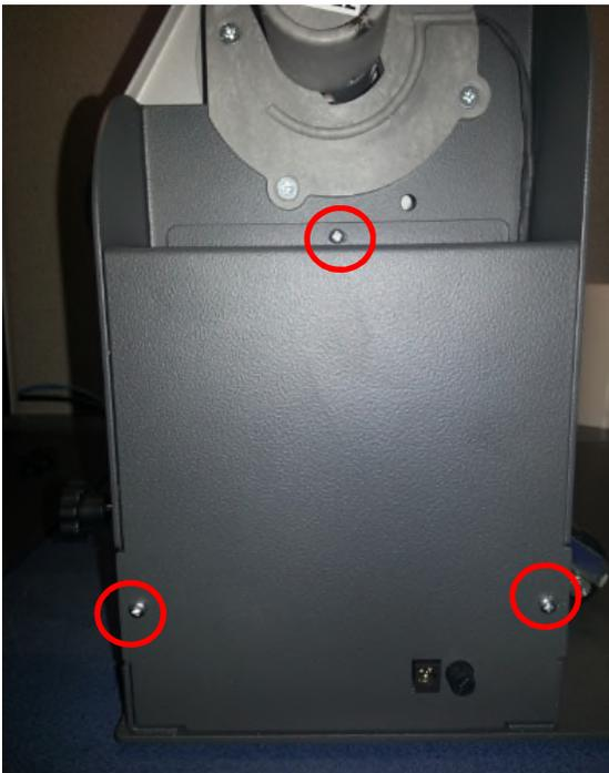
3. Once the screws have been removed, remove the plate
