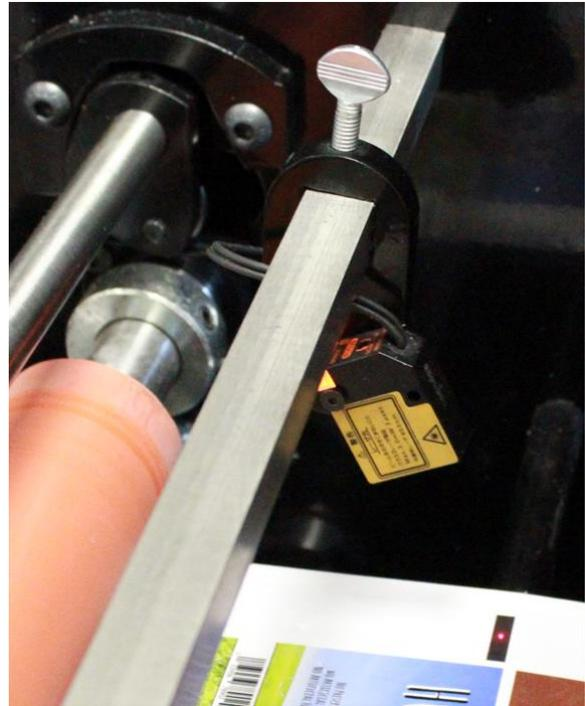
**TIP:** If you do not adjust the collars towards the back of the press and regularly place the registration mark at the same position in your artwork, the position of the sensor should not need to be changed.
