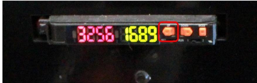
3. Manually move the media a little forward so the laser is pointing onto the media color only.
