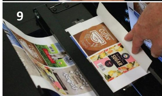
**Note:** The printed images do not need to splice together perfectly, but you will need to perform a **Home Cycle** when the splice gets to the cutting cylinder.
