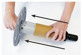
**STEP 2**Load the cardboard core onto the core holder.
