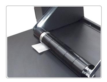
**STEP 2**Put a piece of paper between the aluminium ring and the screw on the basement.
